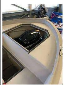
A lot of the time the petrol tank and filter connections are also placed in this same engine bun, the bun will thus house the petrol tank, outboard engine and all relevant assembly fittings including filters and hoses. Such an installation thus has all the characteristics of a petrol inboard engine as the compartment is closed during sailing.
