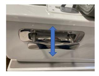
Are pull-out devices like the above-shown deemed to be handholds if installed according to the location and strength requirements as per chapter 9 of EN ISO 15085?
